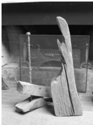
Two hull support pieces from the "White Oak" schooner, built in Oakville.
